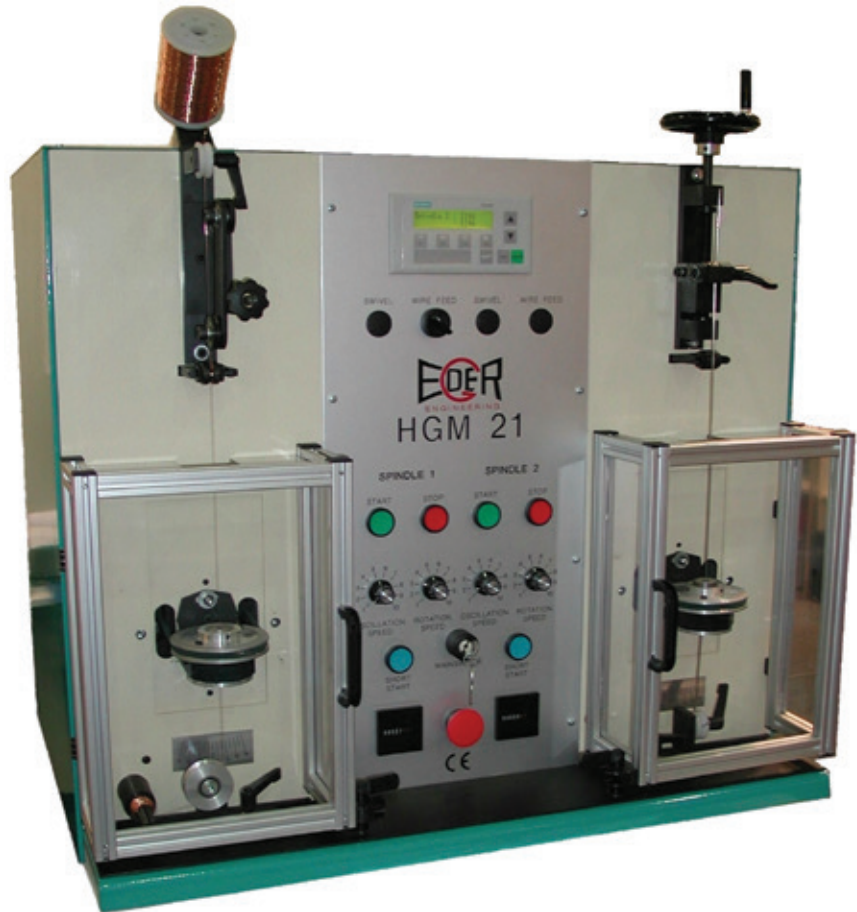
▲ HGM-21 high-speed wire type calibration unit for sizing and polishing of cylindrical die bearings
